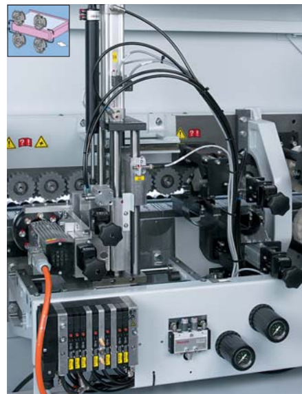
Corner rounding unit Optimum corner rounding without adjustment or set-up, resulting from the coupled diamond tool and tracer roller.
